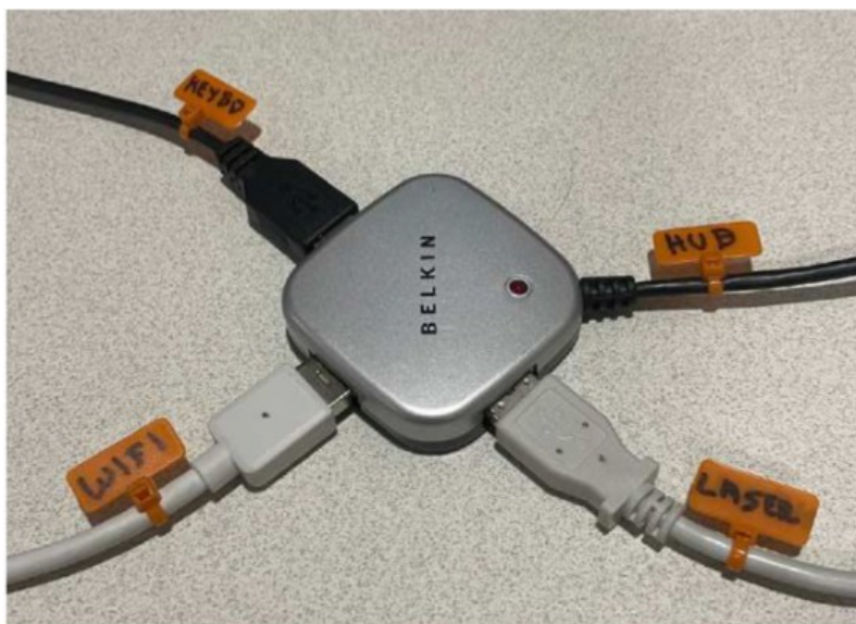
Figure 3 — Tagged zip ties being used as wire labels on the USB hub. [Ray Fallen, ND8L, photo]
