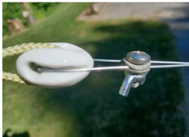
Figure 4 — A screw and two flat washers let you easily adjust the length of a wire antenna. [Paul Conaway, KD2DO, photo]
