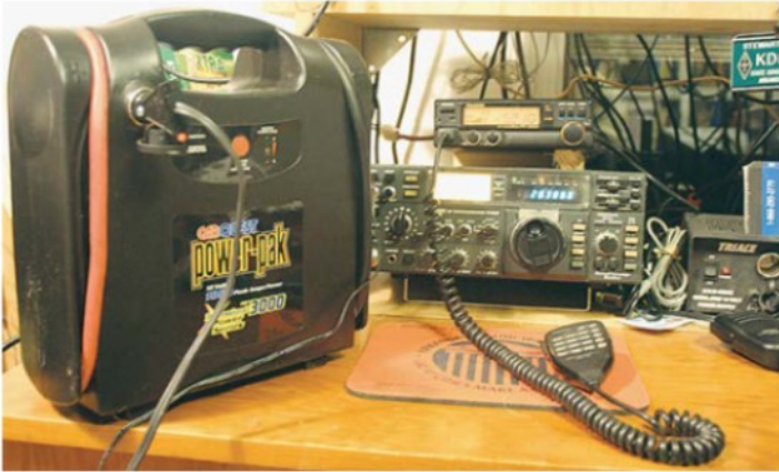
Emergency power supply running a VHF transceiver.
