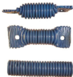
Top image is a side view of a finished insulator, and middle image is a top view. At the bottom is a piece of PVC conduit used for construction of the insulator.
