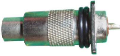
Simple O-rings slipped on to an SO-239 can help create a weather-tight seal.
