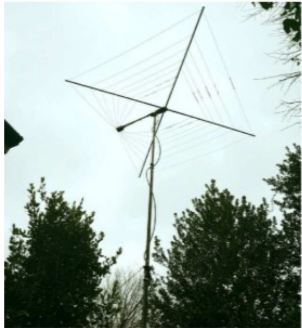
Figure 2 — David Webber's, G0PBS, cobweb antenna. A cobweb antenna is a fan dipole that is wrapped on itself. It is a compromise antenna. One compromise is that for any given band, it doesn't cover the entire band and must be tuned to cover the part of the band that is desired. Another compromise is that the gain is 2 or 3 dB less than an equivalent dipole. Because the antenna is built upon the idea of a dipole, it is a balanced antenna, and radials are not required. [David Webber, G0PBS, photo]
