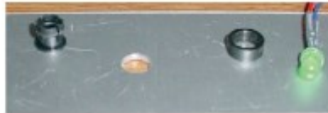
Figure 2 (right): Press-on mounts make it easy to install LEDs in a faceplate.
