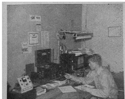
David Langley, of Auroras, N. C., at the controls of W4YDY. The transmitter is a Harvey-Wells Deluxe, with fifty watts input on the 3.7-Mc. band. The receiver is an SX-71. Dave made his first contact last Christmas day.
