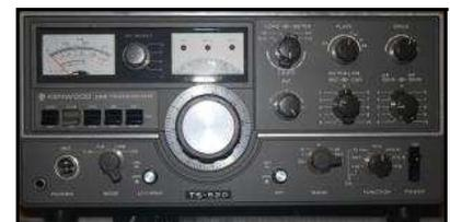
ham bands. It also features receive of WWV at 10 MHz. The TS-520 features a very accurate linear analog display dial. Power input is 120W PEP SSB and 100W CW. (This transceiver does not have general coverage receive). The hybrid circuit includes three 6146A and two 12BY7A tubes plus 1 IC, 17 FETS, 45 transistors and 84 diodes. **REDUCED \$185 or best offer. Contact W4JNC, campbellerecu@embarqmail.com** (Phone 758-1244)
