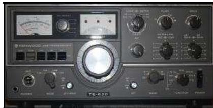
and CW modes in the 80 through 10 meter ham bands. It also features receive of WWV at 10 MHz. The TS-520 features a very accurate linear analog display dial. Power input is 120W PEP SSB and 100W DC CW. (This transceiver does not have general coverage receive). The hybrid circuit includes three 6146A and two 12BY7A tubes plus 1 IC, 17 FETS, 45 transistors and 84 diodes. **\$350 or best offer. Contact W4JNC, president @ w4amc.com.** (Phone number below)
