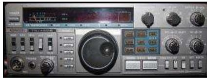
SSB, CW, AM and FM (optional) modes. Coverage is 160 through 10 meters including the WARC bands. All solid-state technology is input rated at 250 PEP on SSB, 200W DC on CW, 120W FM (optional) and 60W AM. General coverage receive from 150 kHz to 30 MHz is featured. **\$350 or best offer.**
