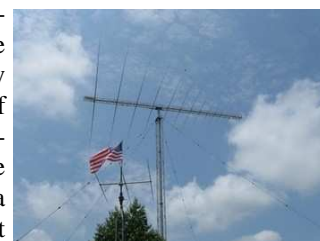
Sixteen element log periodic antenna next to the BARC Field Day site.
