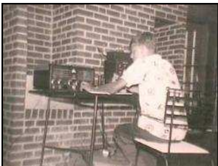
My Hallicrafters SX-71 and Harvey-Wells TBS50D set up on a back screen porch in Florida while on vacation in July 1953. Antenna was a 300 ohm folded dipole and matching balun coils sit on top of transmitter.
